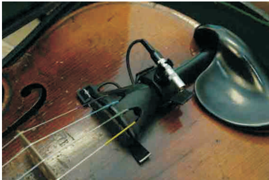
Picture 2: Contact mic connector clipped onto tailpiece cradle.
