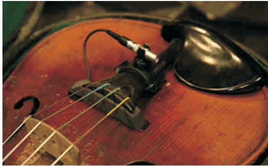
Picture 1: Contact Microphone under tailpiece.
